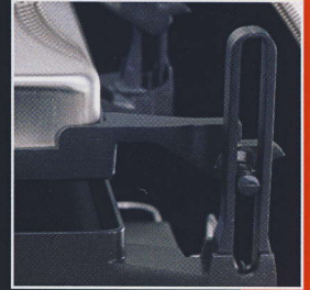
Self adjusting height of top plate
